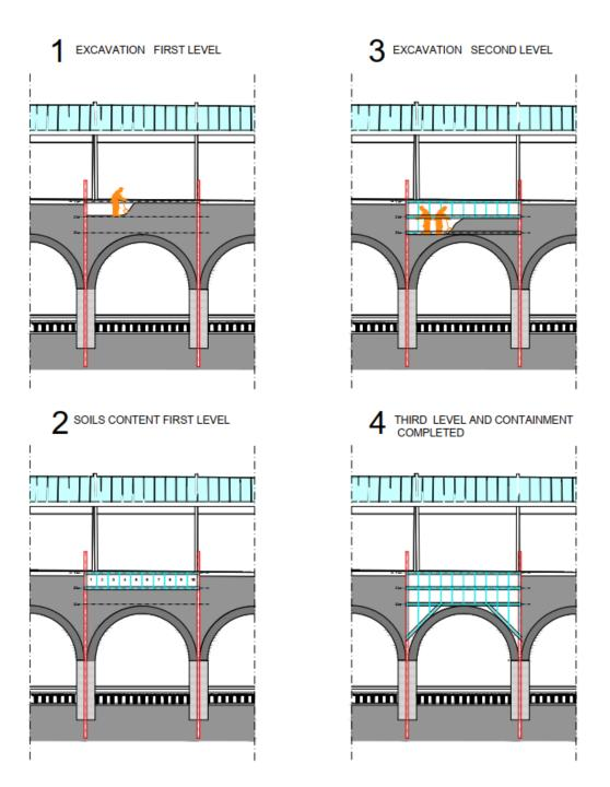
Figure 58. Excavation phases and soils contain between platforms.
