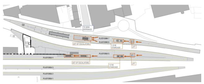
Figure 17. Platform facilities. Proposed additional means of access to the platforms
