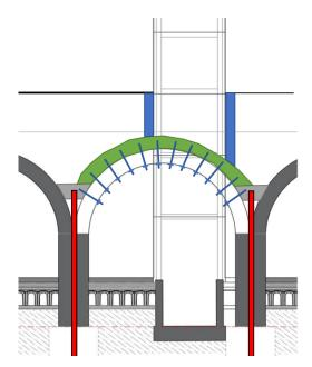
Figure 47. Sketch showing the structural solution for a void containing a lift
