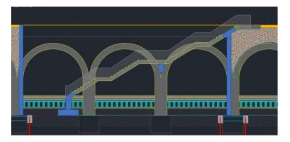
Figure 46. Sketch showing the structural solution for a void containing a staircase
