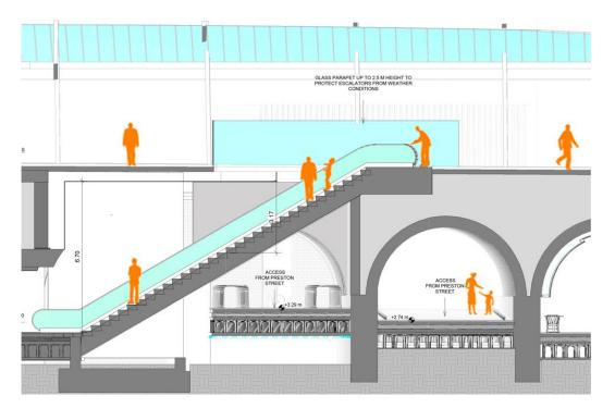
Figure 49. Section of the analysed escalator and opening
