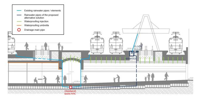
Figure 69 – Rainwater drainage system. Proposed solution
