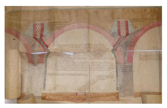
Figure 31. Section drawing of the vaults drainage original project
