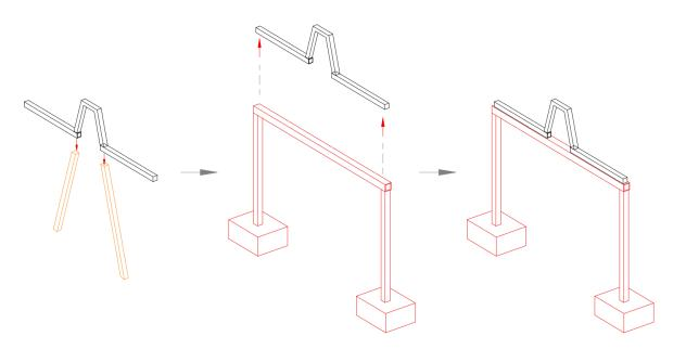
Figure 53. Cut of the existing structure. New steel structure and foundations on platform.
