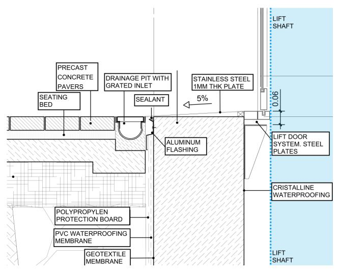
Figure 36. Waterproofing lift detail example that will be adapted to the details of the project
