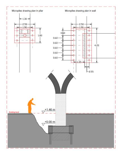
Figure 51. Elevation drawing of excavation up to base of pile cap. Plan drawing of two types of foundations.
