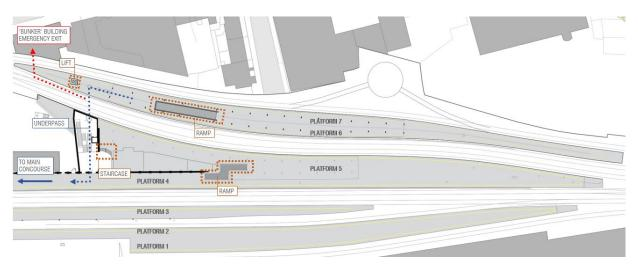
Figure 15. Platform facilities. Existing means of access to the platforms.
