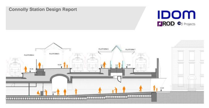
Figure 22. Section through the entrance vault that connects Preston Street with the central corridor
