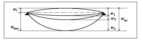
Figure 39 - Definition of vertical deflections. (Source: I.S. EN-1990-2002+A1-2005, A.1.4.)
