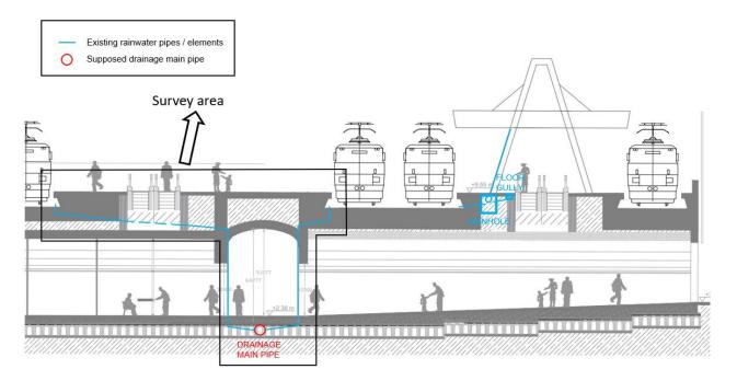
Figure 68 – Rainwater drainage system. Supposed current solution
