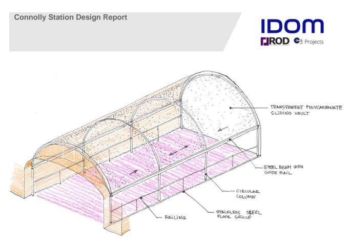
Figure 34. Sketch of the transparent polycarbonate umbrella inside the vault
